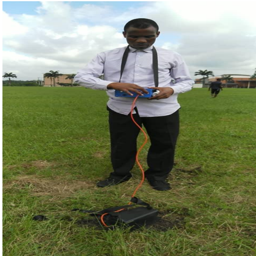
Fig.3: The Compact Digital Terameter (ADMT 200S) cabled to the Rectangular Box-shaped Ground Sensor Used for the VES Resistivity Survey for Detection of Leachate Intrusion into the Aquifer (Field Photograph)
