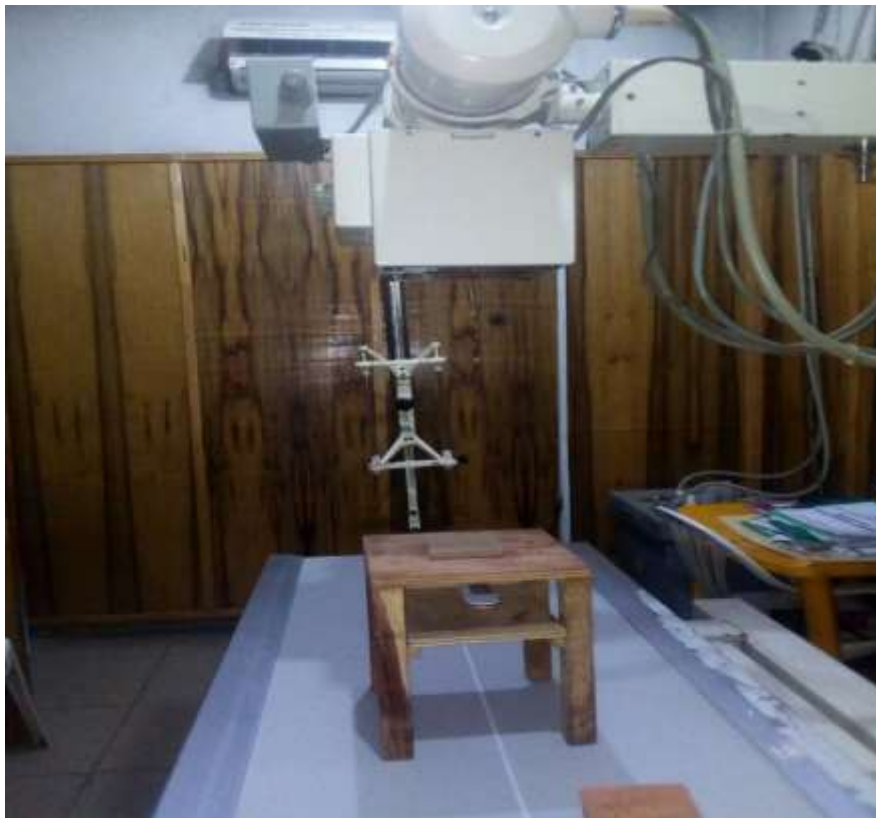
Figure 2: Experimental set up showing the block sample and the radiation detector
