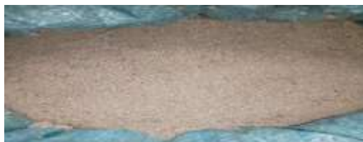
Plate 2.1: Water Hyacinth grinds of size 1.18mm. Plate 2.2: Cassava peelings grinds of size 1.18mm
