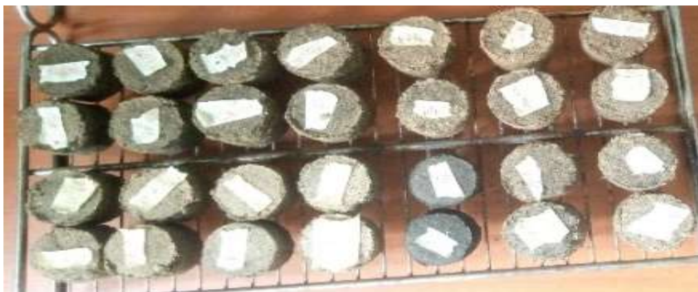
Plate 3.1: Water hyacinth briquettes
