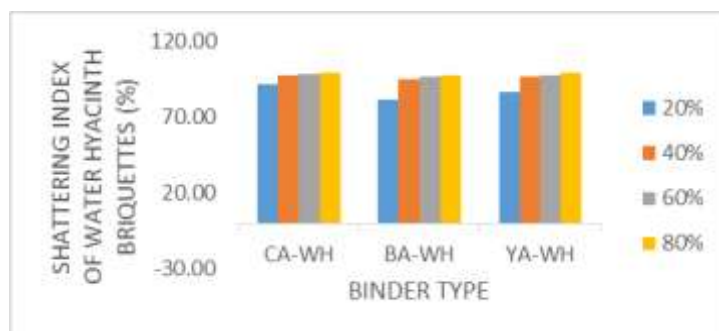
Figure 5 Effect of binder level on the Shattering Index of water hyacinth briquettes
