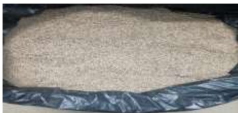
Plate 2.1: Water Hyacinth grinds of size 1.18mm. Plate 2.2: Cassava peelings grinds of size 1.18mm
