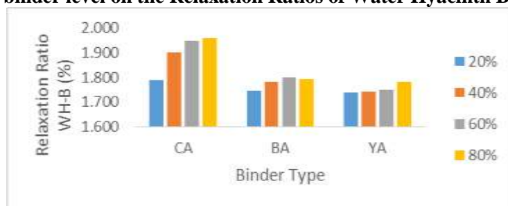
Figure 3: Effect of binder level on Relaxation Ratio
