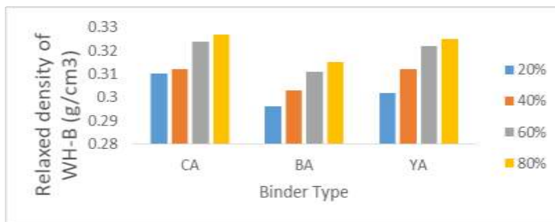
Figure 2: The effect of binder level on relaxed density
