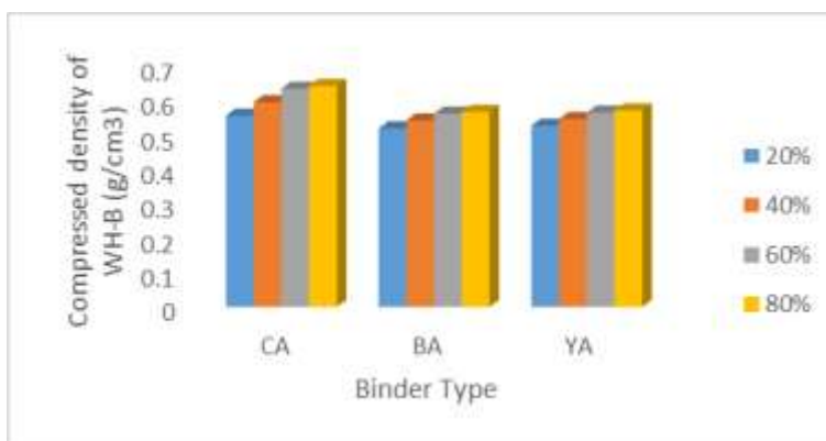
Figure 1: The effect of binder level on compressed density
