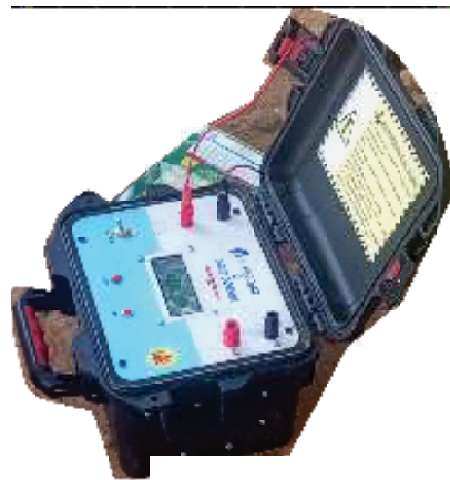
Figure 2c: Omega 48 resistivity meter.
