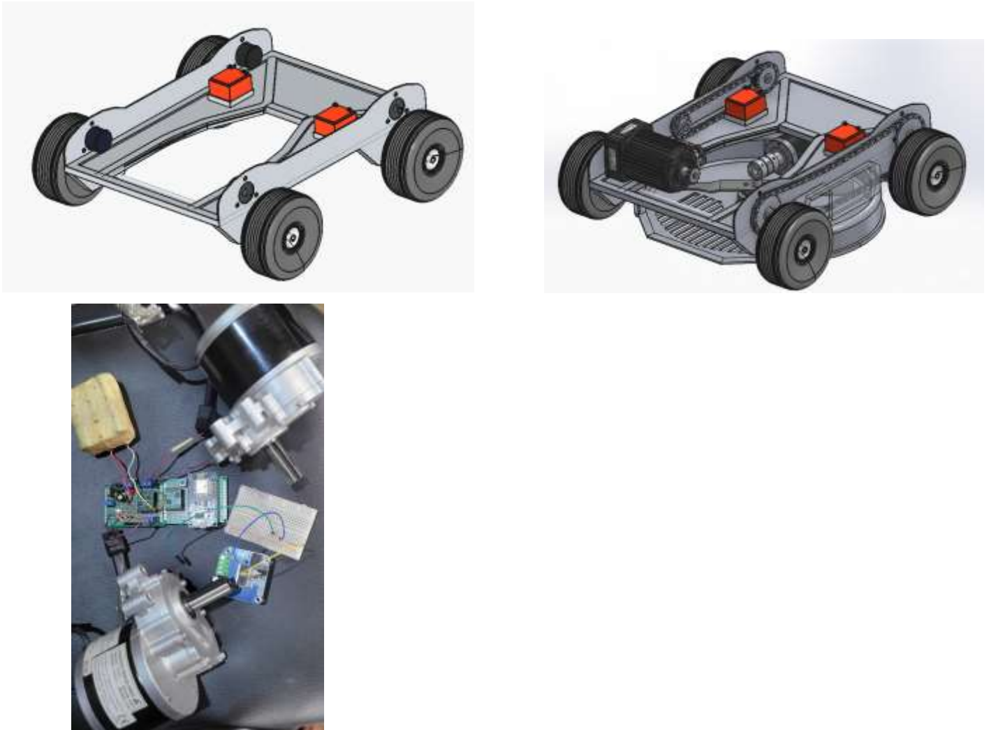
Fig 5: 24V 250W DC motor connected to H-Bridge module for direction and speed control
